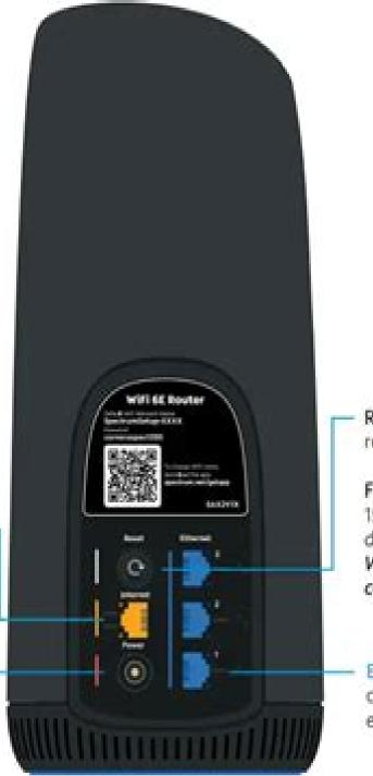
Internet (WAN) port - Connect network cable to the modem for wide area network connection.
