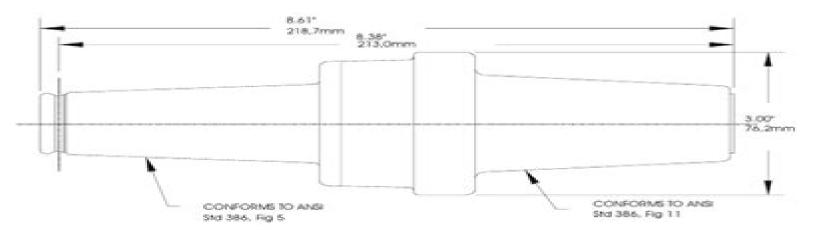
The 15kV 650ETP elbow tap plug permits a 200-amp tap off of a mating 600 Amp connector using load-break elbows. The 650ETP is installed with a 600AT or 600ATM assembly tool.
